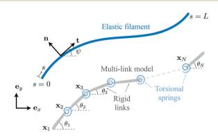
Fig. 5 Schematic diagram illustrating a multi-link discretization of an elastic
