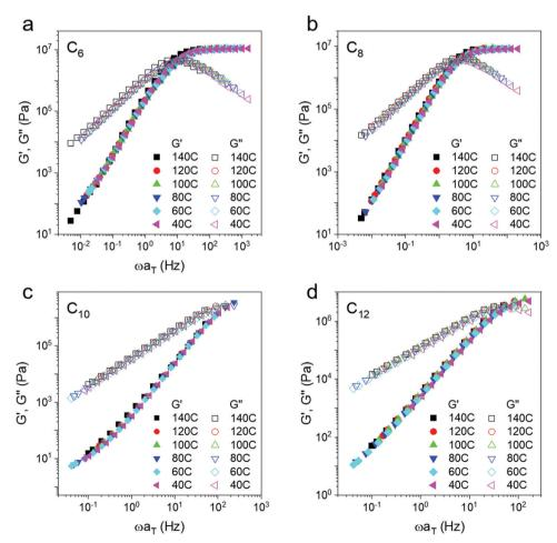
Fig. 3 Horizontally shifted master curves ( $T_{ref} = 140$  °C) of the networks. The high frequency rubbery modulus remains constant with increasing temperature, intermediate to expectations for permanent and dissociative dynamic networks.
