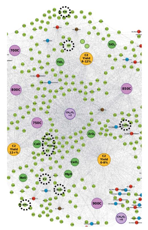
Fig. 4 Locations of element pairs (circled in black) for catalysts EuMgZr-BaO, MoKW-BaO, and KYV-BaO, which are found to have a C<sub>2</sub> yield of 18%.
