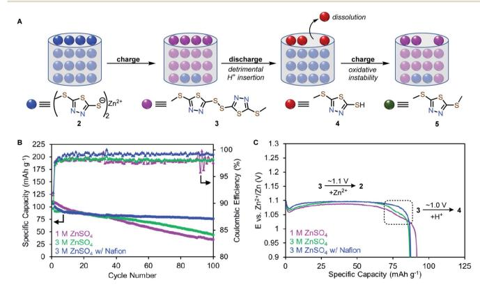
Fig. 6 (A) Qualitative illustration of the decomposition mechanism of 2. (B) Long-term cycling stability and (C) galvanostatic discharge profile (cycle 10) of Zn-2 cells in 1 M ZnSO<sub>4</sub> (purple), 3 M ZnSO<sub>4</sub> (green), and 3 M ZnSO<sub>4</sub> with Nafion (blue).
