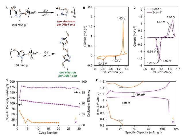
Fig. 3 (A) Oxidation of 1 and 2 to the corresponding disulfides. Solid-state CV measurements of coin cells with (B) 1 and (C) 2 as cathodes and 1 M ZnSO<sub>4</sub> aqueous electrolyte. Counter electrode: Zn. Scan rate:  $0.1 \text{ mV s}^{-1}$ . (D) Galvanostatic cycling comparison of 1 and 2 at a rate of 0.5C. (E) Typical galvanostatic charge–discharge cycling of 1 (orange), 2 (purple), and coulombic efficiency (purple triangle) of Zn-2 cells.
