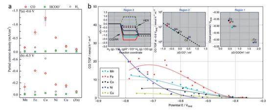
Fig. 1 (a) The volcano trend of M-N-C catalysts in terms of electrochemical  $CO_2RR$  performance. Partial current densities of M-N-C catalysts for CO, HCOO $^-$ , and H $_2$  products at  $-0.6 \text{ V}_{\text{RHE}}$  and  $-0.5 \text{ V}_{\text{RHE}}$ . Reproduced from ref. 56 with permission from the American Chemical Society, copyright 2019. (b) Experimental CO TOFs of M-N-C catalysts. Reproduced from ref. 40 with permission from Springer Nature, copyright 2017.
