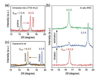
Fig. 4 Structural changes of  $VOPO_4 \cdot nH_2O$  in LiTFSI/4H<sub>2</sub>O. The 001 diffraction peak (a) before and after immersion in LiTFSI/4H<sub>2</sub>O, (b) after lithiation and delithiation in LiTFSI/4H<sub>2</sub>O, and (c) before and after exposure of a lithiated sample to the ambient atmosphere.  $d_{inter}$  denotes the interlayer distance.
