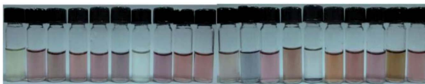
Fig. 7 Optical images of the final GNs solution of AAFQDs in daylight (from left to right: Cys, Ala, Asp, Glu, Phe, Gly, His, Ile, Lys, Leu, Met, Asn, Pro, Gln, Arg, Ser, Thr, Val, Trp, and Tyr). The figure has been reproduced from ref. 93 with permission from Royal Society of Chemistry, copyright 2016.
