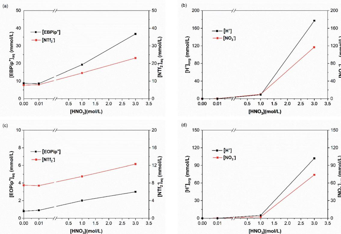
Fig. 5 (a)  $Pip^+$  and  $NTf_2^-$  concentrations in the aqueous phase, (b)  $H^+$  and  $NO_3^-$  concentrations in the organic phase for  $[EBPip^+]$   $[NTf_2^-]$ ; (c)  $Pip^+$  and  $NTf_2^-$  concentrations in the aqueous phase, (d)  $H^+$  and  $NO_3^-$  concentrations in the organic phase for  $[EOPip^+]$   $[NTf_2^-]$ , as a function of the nitric acid concentration, in absence of extractant and metallic cations.
