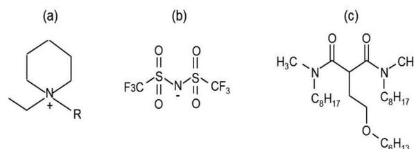
Fig. 1 Chemical structures of the ILs and the extractant used in this work. (a) 1-ethyl-1-alkyl piperidinium cation R = butyl (C<sub>4</sub>H<sub>9</sub>) or octyl (C<sub>8</sub>H<sub>17</sub>) alkyl chain, (b) bistriflimide anion (NTf<sub>2</sub><sup>-</sup>), (c) DMDOHEMA.
