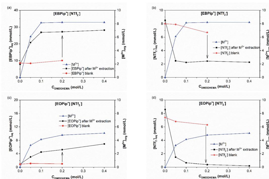
Fig. 7 (a)  $Pip^+$  and (b)  $NTf_2^-$  concentrations in the aqueous phase for  $[EBPip^+][NTf_2^-]$ ; (c)  $Pip^+$  and (d)  $NTf_2^-$  concentrations in the aqueous phase for  $[EOPip^+][NTf_2^-]$ , as a function of the DMDOHEMA concentration and for an initial nitric acid concentration of 0.01 M in the aqueous phase.  $M^{3+}$  is shown on each graph and refers to the total concentration of extracted metal in the organic phase (La, Eu and Fe).
