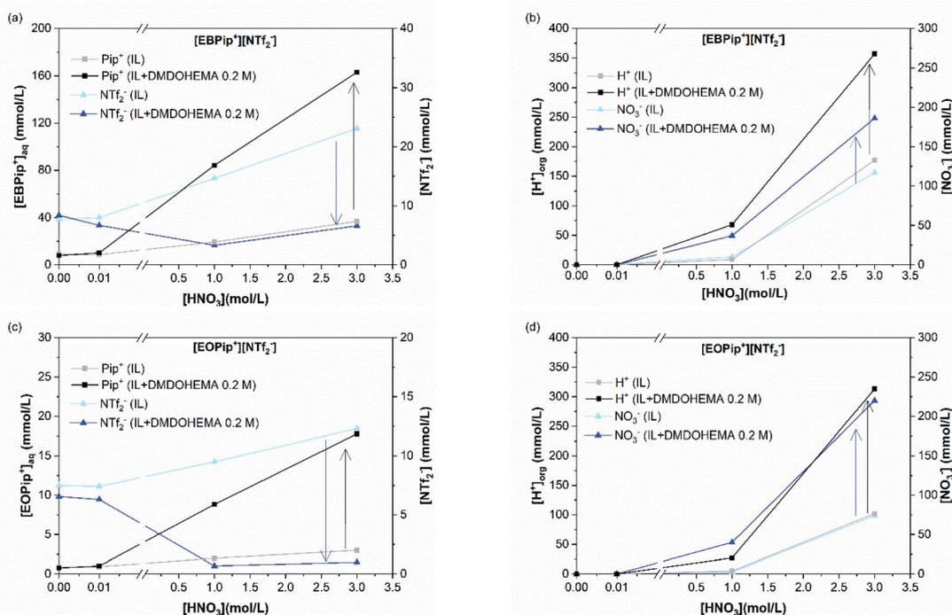
Fig. 6 (a)  $\text{Pip}^+$  and  $\text{NTf}_2^-$  concentrations in the aqueous phase, (b)  $\text{H}^+$  and  $\text{NO}_3^-$  concentrations in the organic phase for  $[\text{EBPip}^+][\text{NTf}_2^-]$ ; (c)  $\text{Pip}^+$  and  $\text{NTf}_2^-$  concentrations in the aqueous phase, (d)  $\text{H}^+$  and  $\text{NO}_3^-$  concentrations in the organic phase for  $[\text{EOPip}^+][\text{NTf}_2^-]$ , as a function of the nitric acid concentration, without and with DMDOHEMA 0.2 M.
