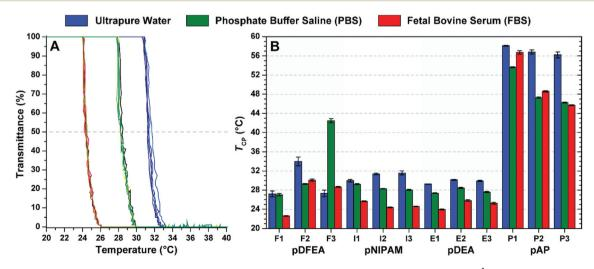
Fig. 3 (A) Comparison of 6 turbidimetric measurements of I2 (pNIPAM) in water, PBS and FBS ( $c = 10.0 \text{ mg mL}^{-1}$ ); (B)  $T_{CP}$  of all polymers in water, PBS and FBS ( $c = 10.0 \text{ mg mL}^{-1}$ ) expressed as a mean of 6 measurements  $\pm$  standard deviation. The results indicate a shift in  $T_{\text{CP}}$ .
