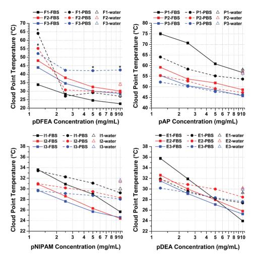
Fig. 4 Plot of  $T_{CPS}$  of the polymers pDFEA (top-left), pAP (top-right), pNIPAM (bottom-left) and pDEA (bottom-right) in FBS and PBS as a function of polymer concentrations. All  $T_{CPS}$  are expressed as the mean of 6 measurement cycles  $\pm$  standard deviation. Asterisks (\*) indicate potential outliers.
