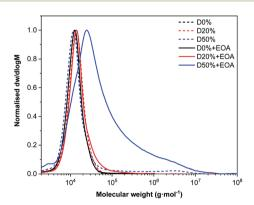
Fig. 4 Normalised SEC RI molecular weight distributions (THF + 2% v/v NEt<sub>3</sub>, 40 °C, PS standards) of D0%, D20%, and, D50% and before and after treatment with EOA and purification by dialysis.
