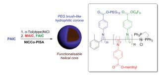
Scheme 1 NiCCo-PISA to prepare functional P(PAIC)<sub>20</sub>-b-(P(MAIC)<sub>x</sub>co-P(FAIC)<sub>v</sub>)<sub>30</sub> diblock copolymer nano-objects.
