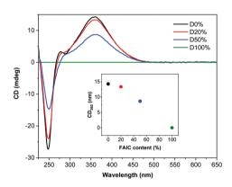
Fig. 3 CD (THF, 0.5 mg mL<sup>-1</sup>) spectra of  $P(PAIC)_{20}$ -b- $(P(MAIC)_y$ -co-P $(FAIC)_z)_{30}$  with 0, 20, 50 and 100 mol% of FAIC.
