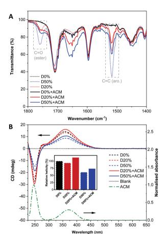
Fig. 8 (A) FT-IR and (B) CD (THF, 0.5 mg mL<sup>-1</sup>) spectra of the D0% (black), D20% (red) and D50% (blue) copolymers before (dotted lines) and after PPM with ACM (solid lines). UV/Vis spectrum (THF, 0.5 mg mL<sup>-1</sup>) of free ACM. The inset shows the helicity (CD at  $\lambda$  = 360 nm) of the copolymers compared to D0%.
