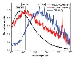
Fig. 9 Fluorescence spectra ( $\lambda_{ex}$  = 375 nm) for D50% + ACM and free ACM in THF or H<sub>2</sub>O.
