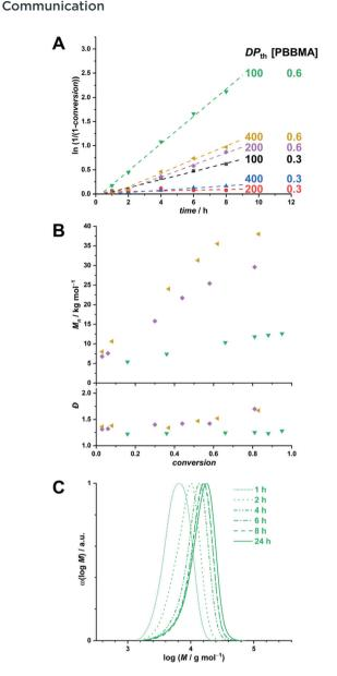
Fig. 1 RAFT solution polymerization of PBBMA in DMAc at 70 °C. (A) First-order kinetic plots for various [PBBMA] and DPth. Dashed lines correspond to linear fits. (B) Evolution of number-average molar mass (top) and dispersity (bottom) with PBBMA conversion for [PBBMA] = 0.6 M at various DPth. (C) Size-exclusion chromatograms of polymers obtained at different times for [PBBMA] = 0.6 M and  $DP_{th} = 100$ .
