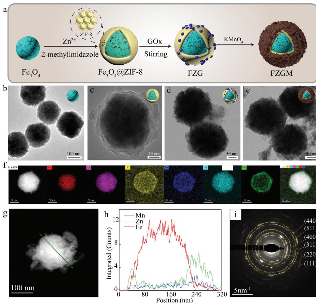
**Fig. 1** (a) Schematic diagram of the fabrication process of the FZGM nanozyme. TEM images of (b)  $\text{Fe}_3\text{O}_4$ , (c)  $\text{Fe}_3\text{O}_4$ @ZIF-8, (d) FZG, and (e) FZGM. (f) HAADF-STEM and elemental mapping images of FZGM. (g and h) Line scan curves of FZGM. (i) SAED diffraction pattern of  $\text{Fe}_3\text{O}_4$ .
