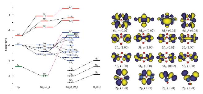
Fig. 4 Kohn-Sham MO analysis of the Np<sub>2</sub>O<sub>3</sub> based on SR-ZORA PBE/TZ2P calculations. The left side is the frontier energy levels, including 6s and 5d bands; the inset on the right side is the  $O_3 \pi^*$  levels.  $Np_2O_3$  orbitals predicted by CASSCF (16, 16) for the nonet state along with the occupation number of orbitals.
