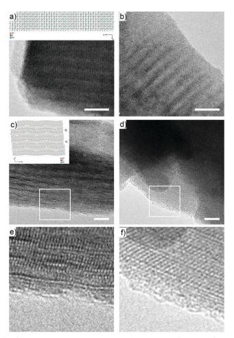
Fig. 2 HR-TEM micrographs obtained for pristine Fk (a, c and e) and Bn-succ-Fk (b, d and f). The insets show the orientations that originate the Moiré pattern in (a and b), and the edge-on perspective of (c and d).<sup>29</sup> Scale bars are 10 nm for a and b and 5 nm for (c and d). (e) and (f) show a zoom in on the edge areas highlighted with white squares in (c) and (d). respectively.
