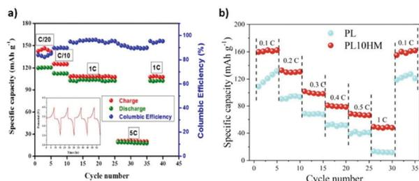
Fig. 11 Rate performance of a Li/Mg-BTC/LiFePO<sub>4</sub> hot pressed cell at 70 °C and corresponding cycling profile<sup>142</sup> (a); rate performance of the PEO/HKUST-1 SPE at 50 °C when compared with a PEO SPE (b).<sup>136</sup>
