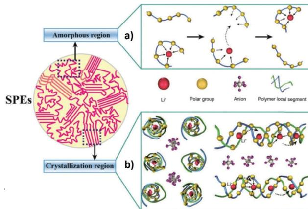
Fig. 6 Schematic illustration of conduction mechanisms in amorphous (a) and crystalline (b) SPEs.<sup>66</sup>
