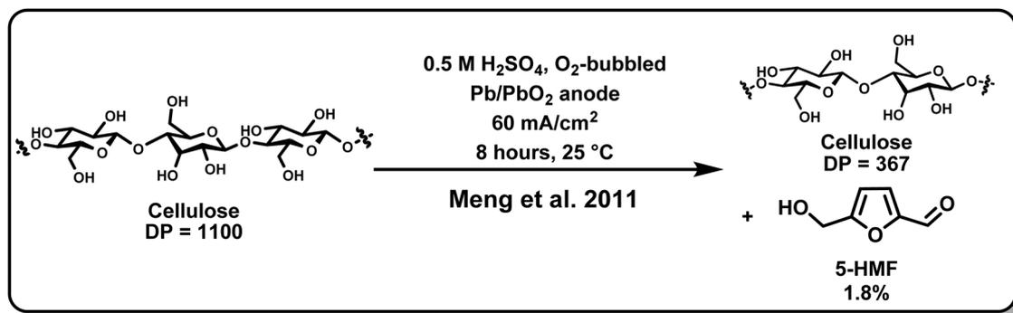
Fig. 4 Electrochemical depolymerization demonstrated by Meng and colleagues.<sup>78</sup>
