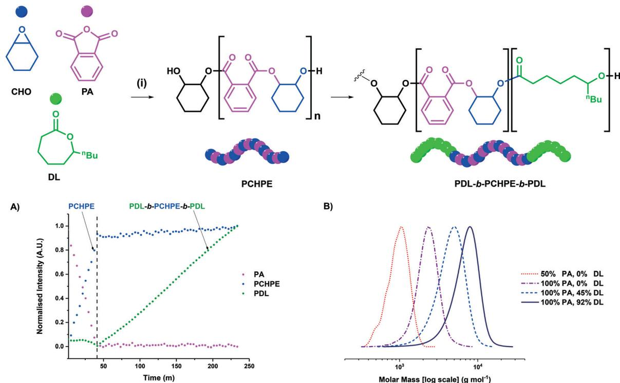
Fig. 3 Switchable polymerization catalysis using PA, CHO and DL utilising complex 1. (i) [Cat]: [PPNCl]: [CHD]: [PA]: [DL]: [CHO] = 1:1:10:100:200:500,  $T = 100$  °C. A) Data from ATR-IR spectroscopy showing the conversion of the different blocks with time. The green series shows formation of PDL, whilst the pink and blue series indicate PA consumption and PCHPE formation, respectively. B) Evolution of polyester molar mass with conversion, from reaction aliquots.
