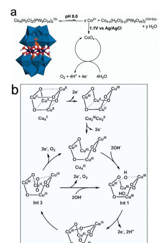
Fig. 6 (a) Heterogeneous CoO<sub>x</sub> formation from homogeneous Co<sub>4</sub>POM. Reproduced with permission from ref. 148. Copyright 2011, The American Chemical Society. (b) Mechanism for the water oxidation of the Cu<sub>4</sub>O<sub>4</sub> core for [(LGly-Cu)<sub>4</sub>]/[(LGlu-Cu)<sub>4</sub>] in alkaline solution. Reproduced with permission from ref. 131. Copyright 2018, Wiley VCH.
