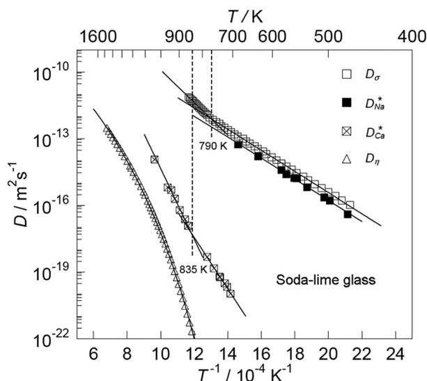
Fig. 8 The temperature-dependent charge diffusion coefficient ( $D_\sigma$ ), tracer diffusion coefficients of  $^{22}\text{Na}$  ( $D_{\text{Na}}^*$ ) and  $^{45}\text{Ca}$  ( $D_{\text{Ca}}^*$ ) and viscosity diffusion coefficient ( $D_\eta$ ) for a soda-lime silicate glass. Reproduced from ref. 63, Copyright (2008), with permission from IOP Publishing.
