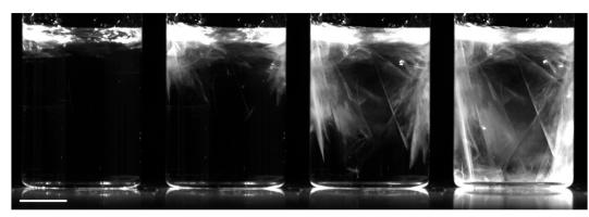
Fig. 4 Nucleation by mechanical shock case (1) where nucleation occurred near the solution-air interface. Images of crystal growth of NaBr (DH) from an aqueous supersaturated solution following nucleation by mechanical shock, from left to right: 3.4, 9, 14, and 19 s after nucleation. Solution conditions:  $C = 10.9 \text{ mol kg}^{-1}$ ,  $T = 21 \,^{\circ}\text{C}$ ,  $S = 1.22 \,(\text{DH})$  or 0.97 (AH). Scale bar represents 5 mm.
