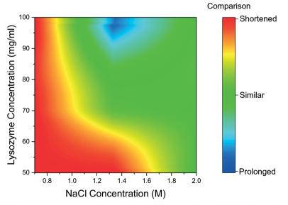
Fig. 5 Contour graph of mean induction times comparison between bubbled droplets and non-bubbled droplets for different conditions.
