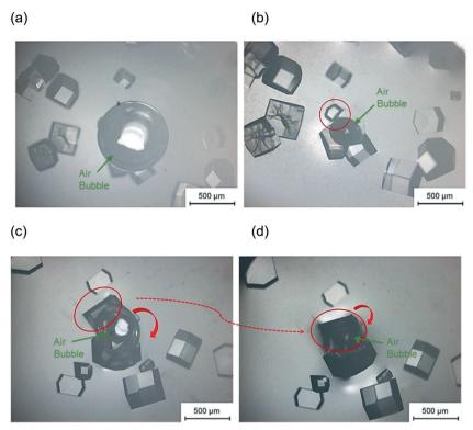
Fig. 3 Microscopic image of a crystal on bubble surface after 6 hours (a) and 55 hours (b) in a hanging drop with condition pH = 4.2, 1.1 M NaCl, and 50 mg mL $^{-1}$  lysozyme and after 77 hours (c) and 140 hours (d) in a different hanging drop with condition pH = 4.2, 1.1 M NaCl, and 70 mg mL<sup>-1</sup> lysozyme.
