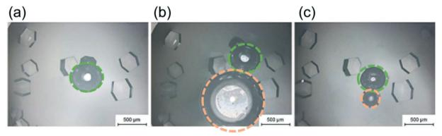
Fig. 4 Effect of second injected bubbles on crystallisation with condition pH = 4.2, 1.1 M NaCl, and 50 mg mL<sup>-1</sup> lysozyme: (a) just before the second bubble injection; (b) immediately after the second bubble injection; (c) 21 hours after the second bubble injection.
