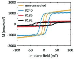
Fig. 9 Comparison of the hysteresis loops for samples #240, #186 and #192 with a non-annealed sample at  $T=100\,\mathrm{K}$ . The non-annealed sample contain a nanocrystalline Fe (11.8 nm) layer and an amorphous Ge (19.4 nm) layer.
