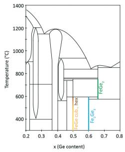
Fig. 1 Fe-Ge temperature-composition phase diagram. Adapted from ref. 37.
