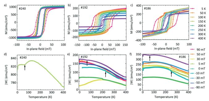
Fig. 8 Magnetic hysteresis curves (a-c) and field-cooling temperature scans (d-f) of samples #240 (left), #192 (center), and #186 (right) in inplane magnetic fields.
