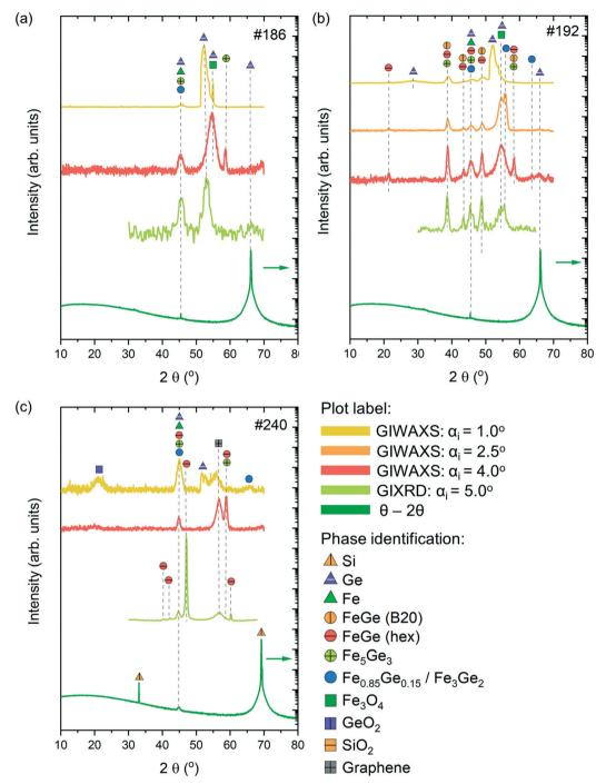
Fig. 6 XRD patterns of (a) #186, (b) #192 and (c) #240 samples measured in GIWAXS (incidence angles  $\alpha_i = 1.0$ , 2.5 and 4°), GIXRD (incidence angle  $\alpha_i = 5.0^\circ$ ) and Bragg-Brentano ( $\theta$ -2 $\theta$ ) configurations, along with the identification of peaks corresponding to different phases. Note that the patterns corresponding to the Bragg-Brentano configuration are presented on the logarithmic scale (pointed with the arrow).
