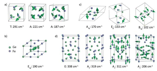
Fig. 4 Representative atomic displacements of the calculated vibrational modes corresponding to a) cubic FeGe phonons at 291, 221 and 187 cm $^{-1}$ , b) hexagonal FeGe phonon at 190 cm $^{-1}$ , c) FeGe $_2$  phonons at 170, 153 and 102 cm $^{-1}$  and d) Fe $_2$ Ge $_3$  phonons at 338, 319, 311 and 206 cm $^{-1}$ . The arrows indicate the direction of displacement, and their sizes show the relative amplitudes of the atomic motions.
