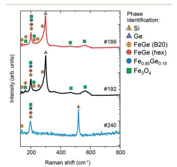
Fig. 7 Raman spectra of #186, #192 and #240 thin films and the comparison with the reference values.
