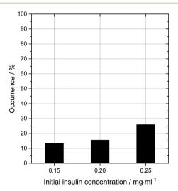
Fig. 4 Occurrence of insulin crystals after 4 days at different initial insulin concentration without amino acids. An initial insulin concentration of 0.2 mg ml $^{-1}$  was chosen as control since the concentration is close to the metastable zone, but still within the nucleation region. The occurrence at this condition is 15.6%.
