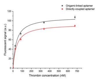
**Fig. 4** One-site binding curves resulting from the measurement of fluorescently labelled thrombin (24–676 nM) for the aptamer linked to the origami structure (black,  $R^2 = 0.98$ ) or the aptamer directly immobilized on the microparticle surface (red,  $R^2 = 0.99$ ). From these data,  $K_D$  values were calculated as the average, obtained from fitting three independent repetitions. Error bars represent one standard deviation (n = 3).
