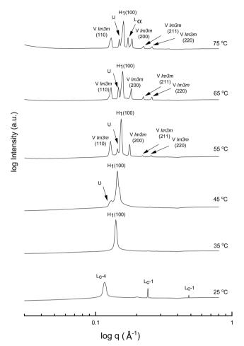
Fig. 3 SAXS patterns of 70 wt% CTAB in water at temperatures between 25 to 75 °C. The liquid crystal phases are denoted as normal hexagonal (H<sub>1</sub>), normal primitive cubic (V<sub>1</sub> ( $Im\bar{3}m$ )), lamellar (L<sub> $\alpha$ </sub>), and unassigned transient (U) liquid crystal phases. The symbols  $L_c$ -1 and  $L_c$ -4 denote lamellar surfactant crystalline phases.
