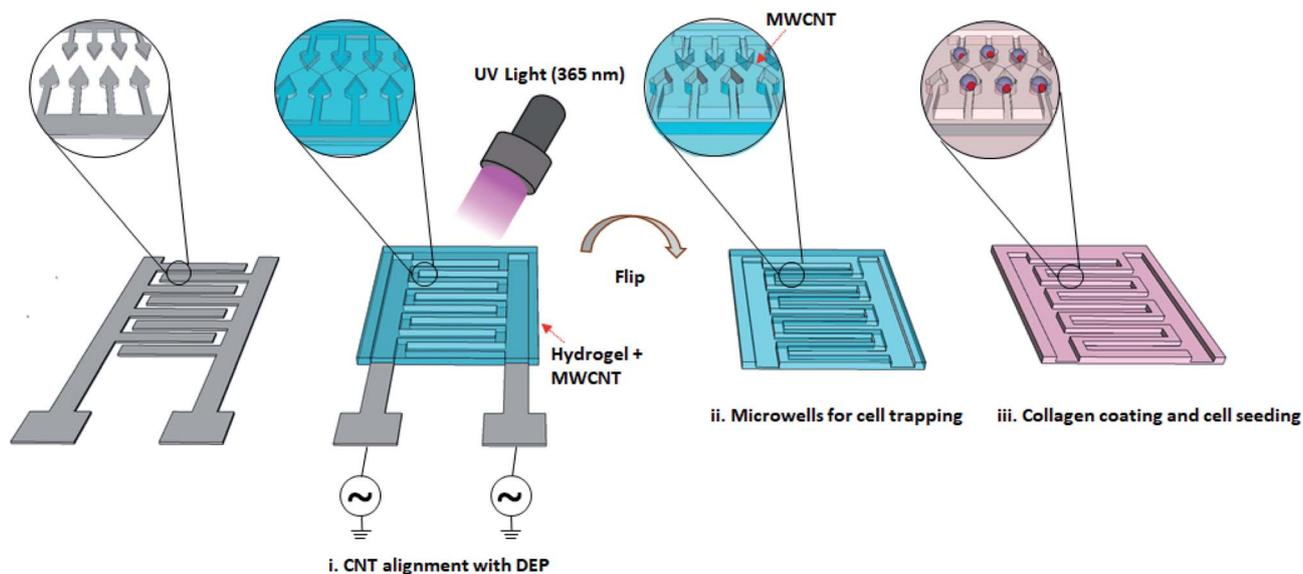
**Fig. 1** A schematic illustration of the strategy used to align and fix MWCNTs in PEGDMA. CNTs were aligned in PEGDMA on an IDA chip using DEP and then fixed via UV crosslinking. The gel with aligned CNTs was peeled off, flipped and placed in a culture dish. After coating the entire surface with collagen, PC12 cells were seeded on the gel and cultured for 24 h at 37 °C. The next day, NGF was added to the medium to induce neuronal differentiation.
