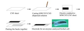
**Scheme 1** Schematic illustration of electrode preparation for the enzyme-catalyzed biofuel cell.
