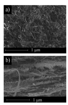
Fig. 3 SEM images of the surface (a) and cross section (b) of the MWCNT/CNF sheet.
