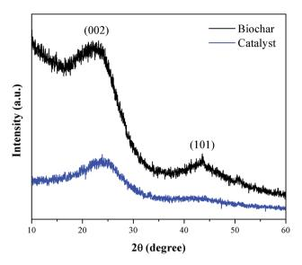
Fig. 3 XRD diffraction patterns of biochar and catalyst.
