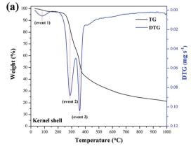
Fig. 7 TGA/DTG curves of (a) kernel shell and (b) biochar.
