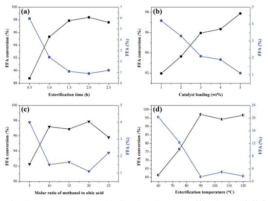
Fig. 9 Influence of esterification parameters on catalytic activity of the sulfonated biochar catalyst. (a) Esterification time (at  $90 \,^{\circ}$ C with the molar ratio of methanol to oleic acid of 20 : 1 and catalyst load of  $5 \,^{\circ}$ C with the molar ratio of methanol to oleic acid of 20 : 1), (c) methanol/oleic acid molar ratio and (d) esterification temperature (for  $1.5 \,^{\circ}$ h with the molar ratio of methanol to oleic acid of 20 : 1 and catalyst load of  $5 \,^{\circ}$ W%).
