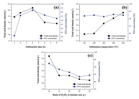
Fig. 2 Influence of sulfonation conditions on the catalytic activity of the sulfonated biochar catalyst (esterification at 90  $^{\circ}$ C for 2 h with the molar ratio of methanol to oleic acid of 20 : 1 and catalyst load of 5 wt%). (a) Sulfonation time (at 200  $^{\circ}$ C and solid-acid ratio of 1 : 10); (b) sulfonation temperature and (at 4 h and solid-acid ratio of 1 : 10); (c) solid-acid ratio of H<sub>2</sub>SO<sub>4</sub> to biochar (at 4 h and 200  $^{\circ}$ C).
