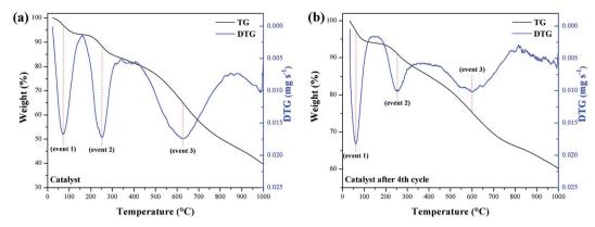
Fig. 8 TGA/DTG curves of (a) catalyst and (b) catalyst reused.
