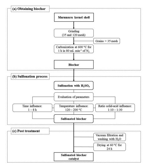
Fig. 1 Scheme of catalyst synthesis process
