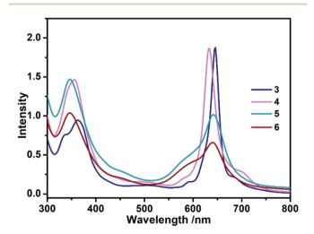
Fig. 1 UV-vis spectra of 3-6 with the concentration of 5.0  $\times$  $10^{-6}$  mol L<sup>-1</sup> in toluene
