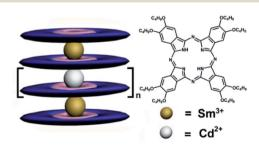
Scheme 1 Schematic molecular structures of tris-to hexakis(phthalocyaninato) metal complexes {[(Pc\*)Sm][(Pc\*)Cd<sub>n</sub>(Pc\*)<sub>n</sub>][Sm(Pc\*)]} (n = 0-3) (3-6).
