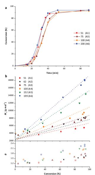
Fig. 5 PEG-X mediated VAc emulsion polymerizations when targeting different DPs for the PVAc block. Evolution of (a) conversion versus time and (b) number-average molar masses  $M_n$  (plain squares) and dispersity  $(D = M_w/M_{pr})$ , hollow squares) with VAc conversion (the dashed lines correspond to the theoretical  $M_n$  values). See Table 1 for details.
