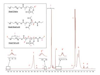
Fig. 2 <sup>1</sup>H NMR spectrum (CDCl<sub>3</sub>, 256 scans) of the dried latex obtained from entry A1. Table 1. after 93% conversion.
