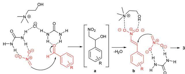
**Scheme 4** Proposed mechanism for the Henry reaction in the DES ChCl/urea.<sup>18</sup> The  $\beta$ -nitro alcohol **a** intermediate is dehydrated to the  $\beta$ -nitrostyrene **b** which undergoes a Michael addition of a nitronate ion.
