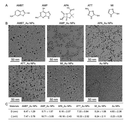
Fig. 2 The morphology, size, dispersity, and zeta potential of the N\_Au NPs. (A) The structure of N-heterocyclic molecules. (B) TEM images of the Au NPs. (C) DLS analysis results of the N\_Au NPs.
