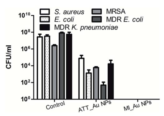
Fig. 6 Antibacterial activity of ATT\_Au NP and MI\_Au NP coated fabrics. Control designates uncoated fabrics. The results represent the average of three independent experiments.
