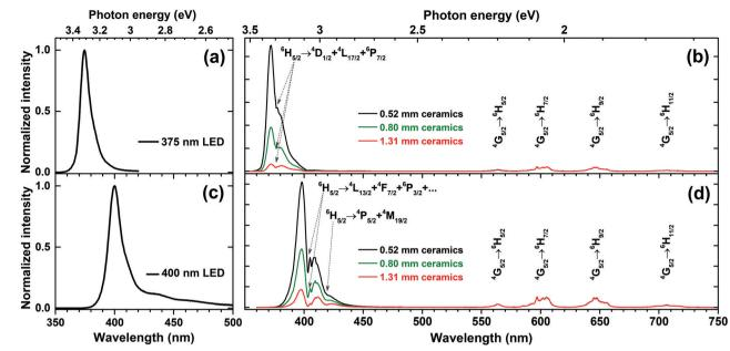
Fig. 8 Emission spectra of (a) 375 nm LED, (c) 400 nm LED. Emission spectra of  $K_2Bi(PO_4)(MoO_4)$ :5%Sm<sup>3+</sup> ceramic discs excited with (b) 375 nm LED, and (d) 400 nm LED.
