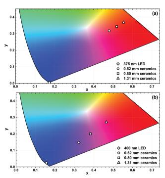
Fig. 9 Fragments of the CIE 1931 colour space diagram with colour coordinates of  $K_2Bi(PO_4)(MoO_4)$ :5%Sm³+ ceramic disks combined with 375 nm (a) and 400 nm (b) emitting LEDs.
