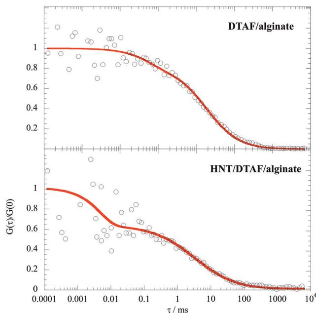
**Fig. 7** Normalized FCS decay curves for DTAF/alginate and HNT/DTAF/alginate mixtures in water. The concentration of DTAF/alginate was set at  $0.1 \text{ mg dm}^{-3}$ , while the overall concentration of alginate was fixed at  $10 \text{ g dm}^{-3}$ . Accordingly, the labelled alginate/HNT mass ratio was  $10^{-4}$  and the mass ratio between the overall alginate and HNT was 0.1. Red lines represent the fitting according to the triplet state model.<sup>56</sup>
