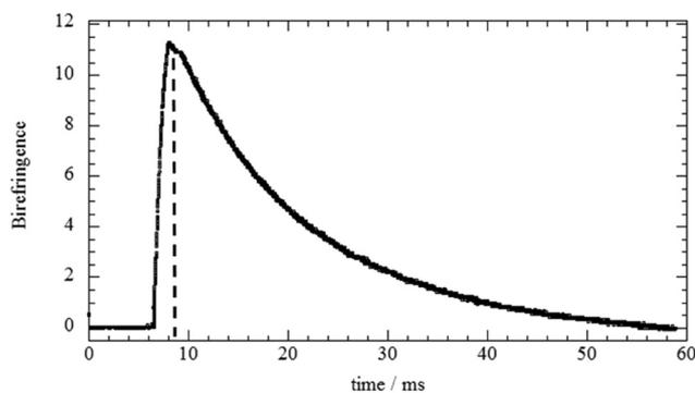
**Fig. 4** Transient electric-field-induced birefringence signal for aqueous dispersion with a HPC/HNT mass ratio of 0.1. The HNT concentration was  $0.15 \text{ g dm}^{-3}$ . The experiments were conducted using rectangular pulses (the applied electric field and the pulse length were fixed at  $1.25 \times 10^5 \text{ V m}^{-1}$  and 2.5 ms, respectively). The dashed line represents the time point where the electric field was switched off.
