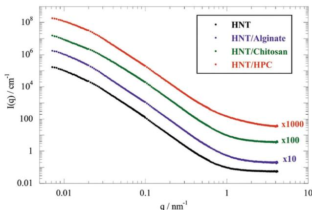
Fig. 1 SANS intensity as a function of  $q$ , the magnitude of the scattering vector, for HNT/chitosan, HNT/alginate, HNT/HPC and HNT dispersions in  $\text{D}_2\text{O}$ . The HNT concentration and the HNT/biopolymer mass ratio were  $80 \text{ g dm}^{-3}$  and 10, respectively.
