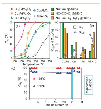
Fig. 3 (a) NO conversion to  $N_2$  during the NO reduction by CO over Pd, Cu, and Cu–Pd catalysts as a function of reaction temperature (NO, CO: 0.5%, GHSV =  $80~000~h^{-1}$ ). (b) Comparison between  $C_{N_2}$  and  $C_{N_2O}$  in NO reduction in the presence of  $O_2$  and  $C_3H_6$ . (c) Stability test for Cu<sub>5</sub>Pd/Al<sub>2</sub>O<sub>3</sub> in the NO + CO reaction at low temperatures (NO, CO: 0.5%, GHSV =  $40~000~h^{-1}$ ).
