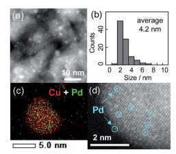
Fig. 1 (a) HAADF-STEM image of  $Cu_5Pd/Al_2O_3$  and (b) size distribution of the nanoparticles. (c) Elemental map of the Pd + Cu overlayer, as acquired by EDS. (d) High-resolution image of a single nanoparticle.
