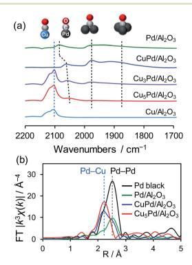
Fig. 2 (a) FT-IR spectra of CO adsorbed on the prepared catalysts. (b) Fourier transforms of the Pd K-edge EXAFS spectra of the Pd-based catalysts.
