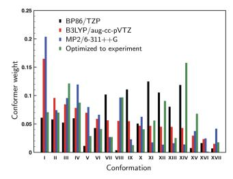
Fig. 2 Computed Boltzmann weights at different levels of theory (black: BP86/TZP; red: B3LYP/aug-cc-pVTZ;<sup>13</sup> blue: MP2/6-311++G<sup>13</sup>). The green weights derive from a fit of the experimental spectrum to the theoretically predicted VCD spectra using conformational weights derived from energies that have been allowed to change freely from their calculated values.
