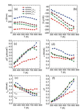
Fig. 8 Temperature dependent (a) electrical conductivity, (b) Seebeck co-efficient, (c) power factor, (d) thermal conductivity, (e) lattice thermal conductivity and (f) thermoelectric figure of merit (zT) for pristine and halogen doped AgPbBiSe3.
