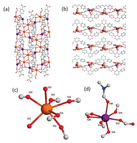
Fig. 2 View of the 2D-sheet structure of MFM-510 along (a) the a-axis and (b) the c-axis. Terminal DMF and water ligands are removed for clarity. View of (c) type I and (d) type II Ba(II) nodes showing trigonal prismatic coordination. H atoms are omitted for clarity. Carbon, grey; oxygen, red; hydrogen, white; nitrogen, blue; barium, orange (type I) and purple (type II).
