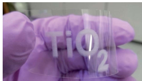
Fig. 7 3-pass " \text{TiO}_2 " print with Ink 2 on a PET substrate.
