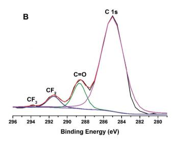
Fig. 8 XPS C1s signals at a takeoff angle of 90 °C; (A) PU and (B) PU-F 3 (1.05 wt%)
