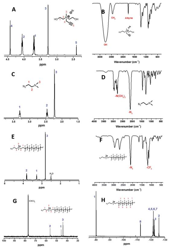
Fig. 2 <sup>1</sup>H NMR and FT-IR spectra of M1 (A and B), M2 (C and D), M3 (E and F) and <sup>13</sup>C/<sup>19</sup>F NMR spectra of M3 (G and H).
