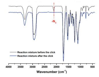
Fig. 5 The FT-IR spectra of reaction mixture containing the PU-Al and M3 before or after the click reaction.
