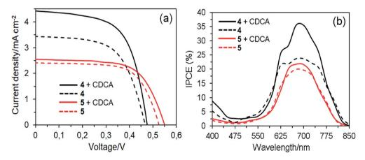
Fig. 10 J-V curves (a) and IPCE spectra (b) of the DSSCs based on dyes 4 and 5 with and without CDCA.
