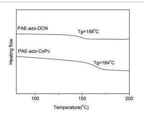
Fig. 5 DSC curves of PAE-azo-DCN and PAE-azo-CoPc.
