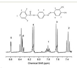
Fig. 2 <sup>1</sup>H NMR spectrum of monomer 2 in DMSO-d<sub>6</sub>.
