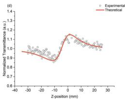
Fig. 8 Z-scan data of (a) PAE-azo-DCN (open aperture), (b) PAE-azo-DCN (close aperture), (c) PAE-azo-CoPc (open aperture), and (d) PAE-azo-CoPc (close aperture).
