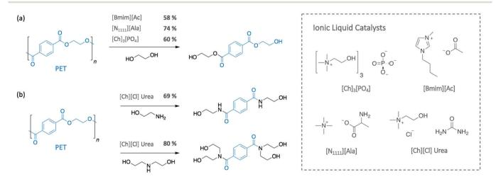
Scheme 2 (a) Glycolysis and (b) aminolysis of PET using different ionic liquids as catalyst.
