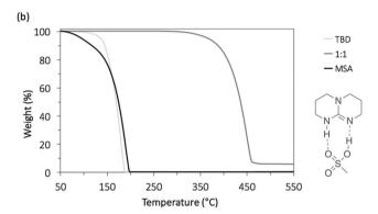
Fig. 4 (a) The depolymerisation of PET and re-polymerisation of monomeric products (BHET) using TBD: MSA (1:1) catalyst and (b) the thermogravimetric analysis (TGA) comparison between TBD: MSA (1:1) and TBD and MSA alone.
