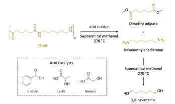
**Scheme 4** Depolymerisation of PA-66 catalysed by organic acids in supercritical methanol.
