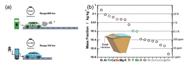
Fig. 1 (a) Refuelling time and charging time of a gasoline car and an electric vehicle, respectively. (b) Elemental abundance in the Earth's crust. Reproduced with permission from ref. 16. Copyright 2014, American Chemical Society.
