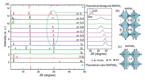
Fig. 1 (a) The XRD spectra of MAPbBr<sub>3</sub> with varying ligand concentration and MAPb(Br<sub>x</sub>l<sub>1-x</sub>)<sub>3</sub> with varying 'Br': 'I' ratio. (b) The primitive cell of cubic-structured MAPbBr<sub>3</sub>. (c) The primitive cell of tetragonal-structured MAPbI<sub>3</sub>.  $L = 15 \mu L$  of ligand (octylamine).
