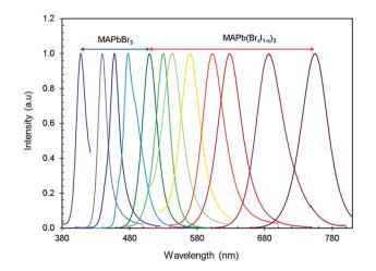
Fig. 4 The normalized PL emission spectra of halide perovskite nanocrystals over the range of 408-755 nm with varying ligand concentration for MAPbBr<sub>3</sub> and composition of 'Br' and 'I' for MAPb(Br<sub>x</sub>I<sub>1-x</sub>)<sub>3</sub>.
