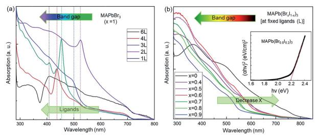
Fig. 3 Optical absorption spectra of (a) MAPbBr<sub>3</sub> with ligand concentration variation and (b) MAPb(Br<sub>x</sub> $l_{1-x}$ )<sub>3</sub> with 'Br' and 'I' composition variation at a fixed ligand amount (1L), and inset is the Tauc plot of the sample at x = 0.8.
