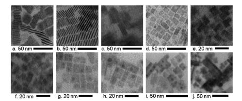
Fig. 2 TEM images of (a-e) MAPbBr<sub>3</sub> with decreasing ligand concentration (4*L*, 3.5*L*, 3*L*, 2*L*, and 1*L*) and (f-j) MAPb(Br<sub>x</sub>l<sub>1-x</sub>)<sub>3</sub> with increasing iodine content (x = 0.8, x = 0.6, x = 0.5, x = 0.4, and x = 0) and fixed ligands (1*L*).
