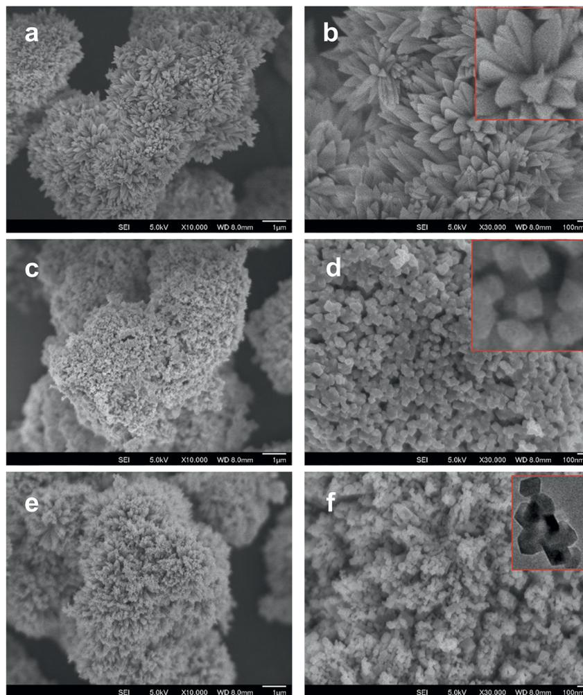
Fig. 2 SEM images: (a and b)  $[\text{Co/Ni}][\text{OH}]_2$ , (c and d)  $\text{Co}_3\text{O}_4/\text{NiO}$ -400 °C, (e and f)  $\text{Co}_3\text{O}_4/\text{NiO}$ -600 °C microsphere composites at low and high magnifications. Scale bars: 1 μm in a, c, e; 100 nm in b, d, f.
