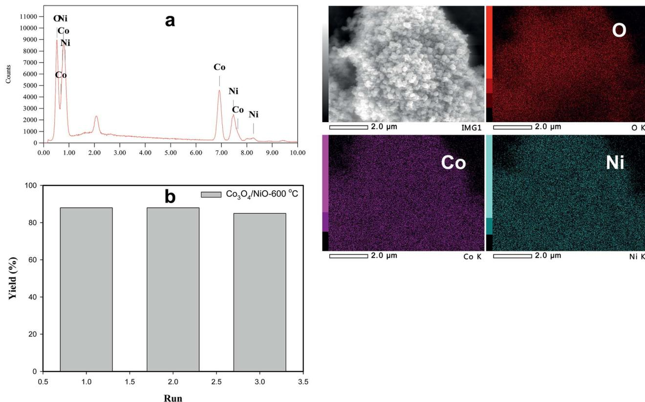
Fig. 8 (a) SEM-EDS spectrum of recycled catalyst; (b) number of run and % yield using recycled Co<sub>3</sub>O<sub>4</sub>/NiO-600 °C microspheres.
