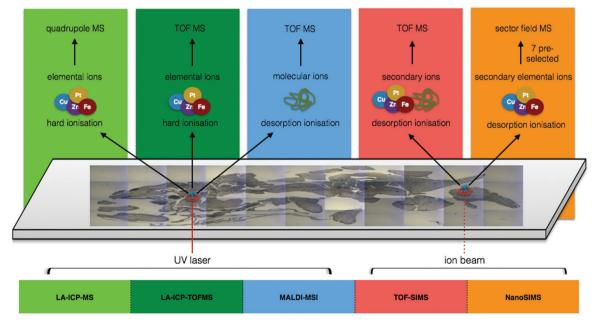
Fig. 5 Comparison of ionisation sources, resulting elemental/molecular ions, and mass detectors among mass spectrometry imaging techniques.
