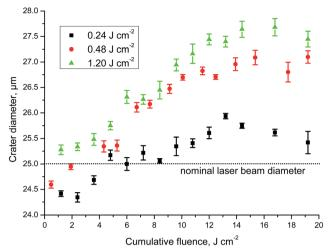
Fig. 4 Assessment of laser ablation crater diameters. Dependence of crater diameter (n = 5) of the reference  $UO_2$  single crystal on the applied cumulative fluence using various fluence levels. The nominal diameter of the ablation crater amounted to 25  $\mu$ m.
