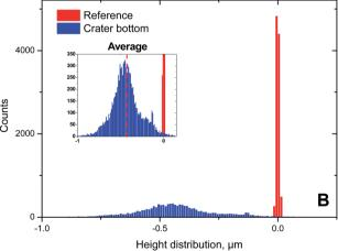
Fig. 3 Characterisation of the laser ablation crater of the reference UO<sub>2</sub> single crystal after 40 laser pulses providing a fluence of 0.24 J cm<sup>-2</sup> each, using a confocal laser scanning profilometer. (A) Representative depth profile of a LA crater. (B) Height distribution of a reference area (red) and of the crater bottom (blue) used to calculate the average step depth. See text for details.
