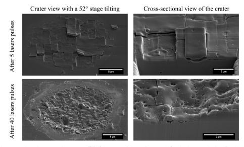
Fig. 2 High-resolution scanning electron microscope (SEM) images of the reference  $UO_2$  single crystal after 5 and 40 laser pulses having a fluence of 0.24 J cm<sup>-2</sup> each. Cross-sectional images of the ablation craters were generated after milling of lateral trenches using a focused ion beam (FIB) microscope.
