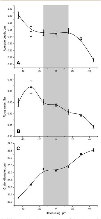
Fig. 5 Influence of laser focus on the average depth, surface roughness and crater diameter as determined on the reference UO2 single crystal. Each data point represents the average of five replicate measurements after application of 40 laser shots having a fluence of 0.24 J cm<sup>-2</sup> each. The grey area represents the laser focus region from -15 μm to +15 μm in which all three investigated parameters remain reasonably constant.
