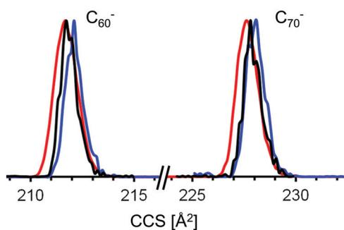
**Fig. 3** Typical mobilograms of  $C_{60}^-$  and  $C_{70}^-$  recorded in the same measurement runs on three different days. Identical colors indicate identical runs. Within the same run, peak maxima can be determined to a relative accuracy of significantly better than 0.5%.<sup>38</sup>
