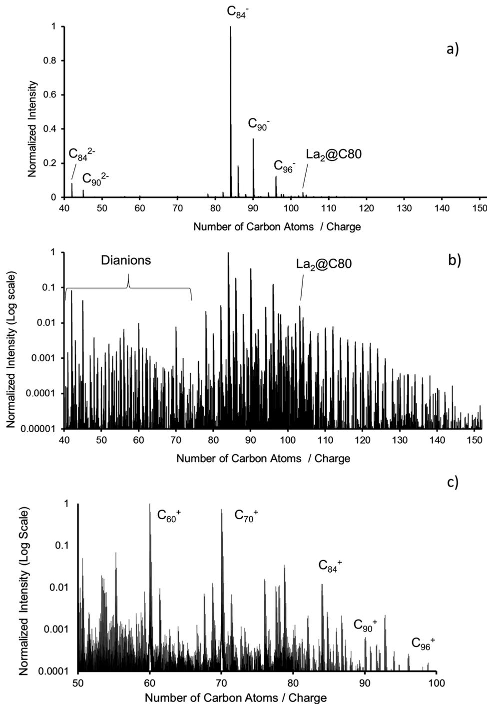
**Fig. 1** Fullerene mix composition. (a) Negative ion ESI-mass spectrum showing  $C_n^-$  and  $C_n^{2-}$  on a linear intensity scale, (b) logarithmic scale, (c) positive ion APCI-mass spectrum showing  $C_n^+$ . The cation mass spectrum is more contaminated, but fullerenes up to  $C_{96}^+$  can be easily identified and their mobilities measured.
