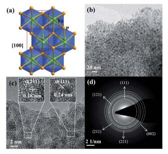
Fig. 6 (a) The crystal structure of FeP crystallizing in the orthorhombic space group  $Pna2_1$  (shown along [100]; the unit cell is shown in red). (b) TEM image displaying homogenously distributed nanoparticles of 2–5 nm in size. (c), HR-TEM image with d-spacing of 0.18 and 0.24 nm (in the inset) corresponding to (211) and (111) planes. (d) SAED pattern exhibiting characteristic rings confirming the phase-purity of FeP (JCPDS 71-2262).
