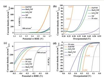
Fig. 7 (a) OER (c) HER polarisation curves of FeP and the benchmark noble metal-based catalysts recorded on NF with a three-electrode configuration in aqueous 1 M KOH electrolyte with a sweep rate of 1 mV s $^{-1}$ . (b) OER (d) HER overpotential comparison of FeP at various (10, 50 and 100 mA (cm) $^{-2}$ ) current densities.
